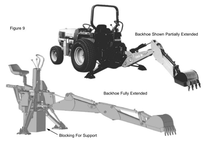
The backhoe is self-assisting during the installation and removal procedures. For removal and storage, follow these steps:
